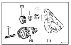
(b) Remove the starter housing (1), idler gear (2), bearing (3), clutch assembly (4) and return spring (5) from the magnetic switch assembly.
